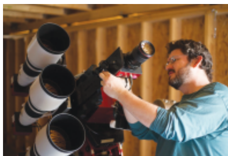
▲ TRIPLED GAZE Roberto Abraham mounts an autoguider camera on the proof-of-concept three-lens prototype.
