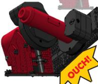
Without a counterweight shaft attached, the RA Axis is out of balance and "top heavy". The above diagram demonstrates what happens when the Two Position Switch is rotated to the Balance Position without the counterweight shaft attached.
