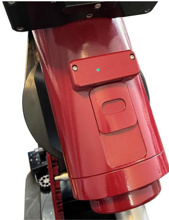
Figure 2: Declination axis with on-axis absolute encoder sensor cover.
