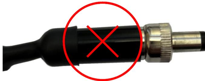
Figure 44: Note that the MKS 5000 PSU plug is *not* compatible with the MKS 6000.
