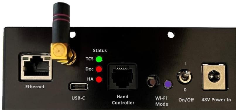
Figure 29: Electronics housing components.
