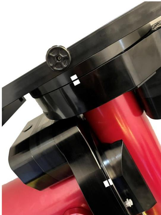
**Figure 9: If you think Find Home is not working, mark the home position on both axes with masking tape as shown.**
