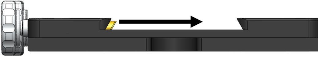
**Figure 19: The brass plunger compresses the male dovetail against the opposite side (from left to right in the above diagram).**
