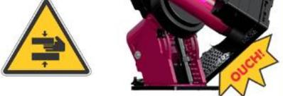
Without a counterweight shaft attached, the RA Axis is out of balance and "top heavy". The above diagram demonstrates what happens when the Two Position Switch is rotated to the Balance Position and the lock knob is in the balance position without the counterweight shaft attached.
