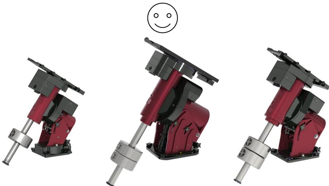
**Figure 67: Before attaching a telescope to the Versa-Plate, orient the Paramount to its “happy place” with the counterweight shaft oriented vertically. In this orientation, the counterweights do not impart any lateral forces on the worm and gear.**
