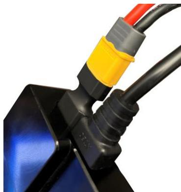
**Figure 54: A female-to-female XT60 extender plugged into the Instrument Panel's Power Port 3.**
