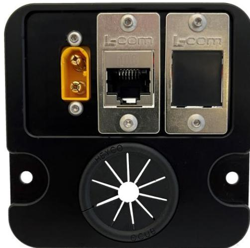
Figure 15: The hour angle axis through-the-mount panel includes one XT60 power input connector, one passthrough Ethernet port and one customizable Keystone module.
