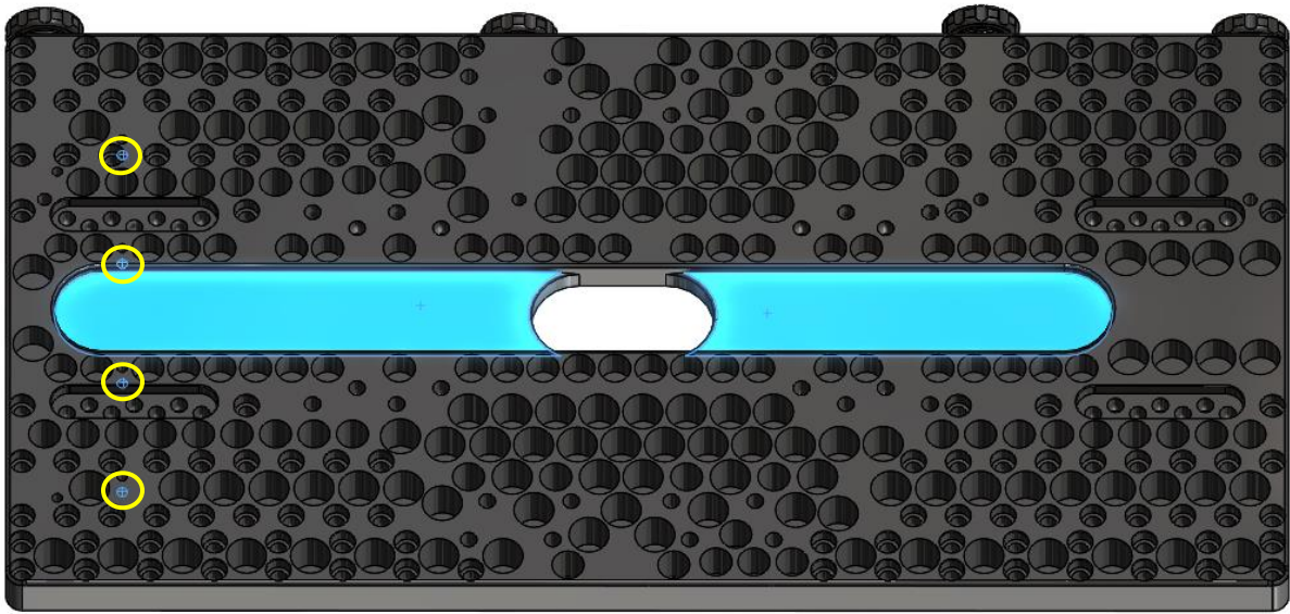
Figure 27: Versa-plate cable channel and instrument panel holes (bottom view).
