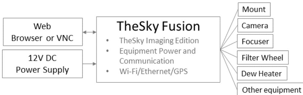
Figure 1: A high-level TheSky Fusion setup diagram.
