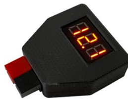
Figure 25: TheSky Fusion DC Voltage Meter showing 12.1V.
