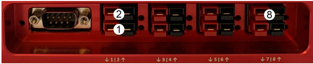
Figure 35: The maximum power supplied by ports 1, 2 and 8 is configurable.
