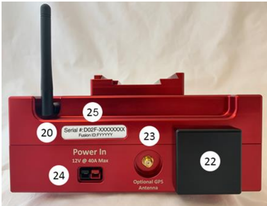
Figure 3: TheSky Fusion rear view with components numbered.
