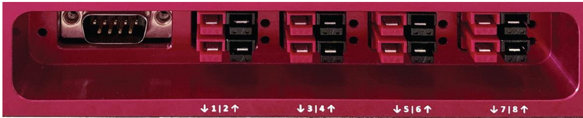
Figure 26: TheSky Fusion's eight power output ports (labeled 1-8).
