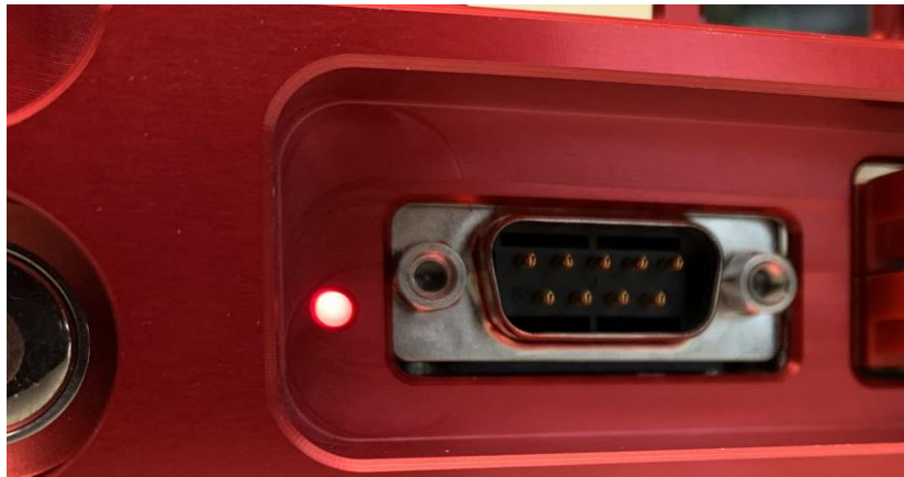
Figure 31: Location of TheSky Fusion's GPS LED.
