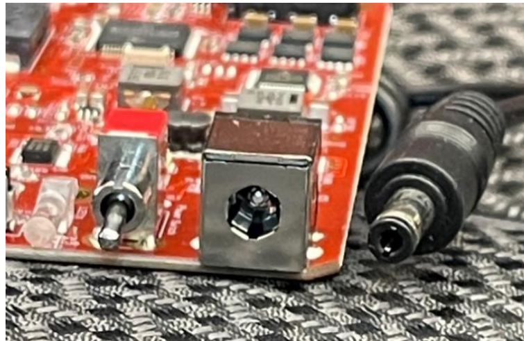
MKS 6000 DC power input jack and power supply connector.
