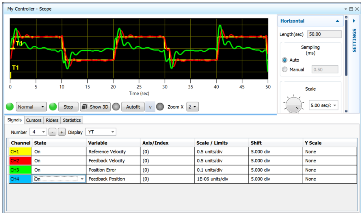
Figure 71: SPiiPlus Scope output giving validity to tuning parameters during a Motion Manager back and forth move. Feedback velocity follows reference velocity and a low, steady-state position error. Note the scale of the position error is 0.1 units/division.
