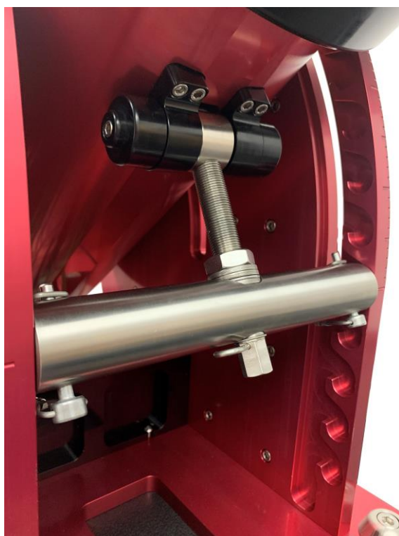
Figure 18: The spring-loaded latitude adjustment bar in slot position 5 (from the bottom of the wedge).
