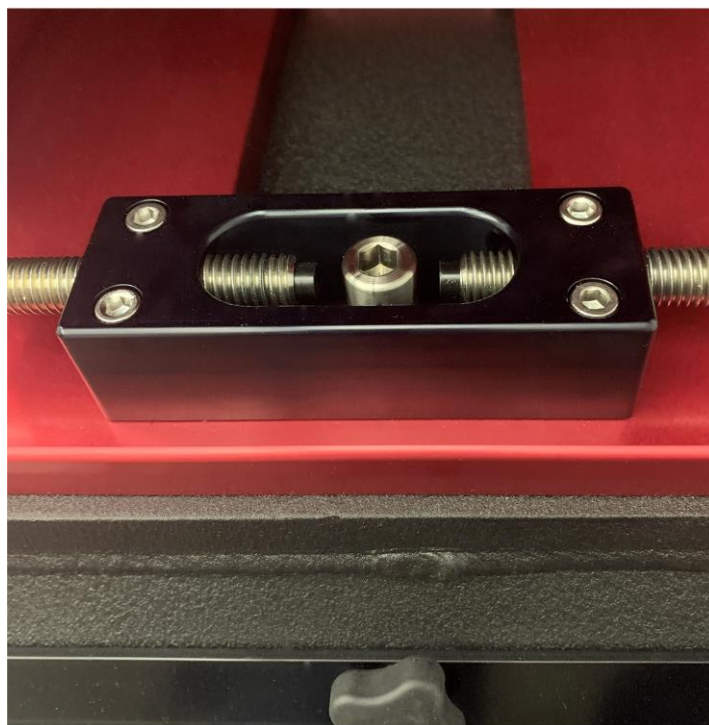
Figure 12: The azimuth adjustment screws must be separated to make room for the azimuth anchor.
