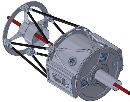
Figure 56: The OTA can be moved along the axis defined by the red line to achieve balance.
