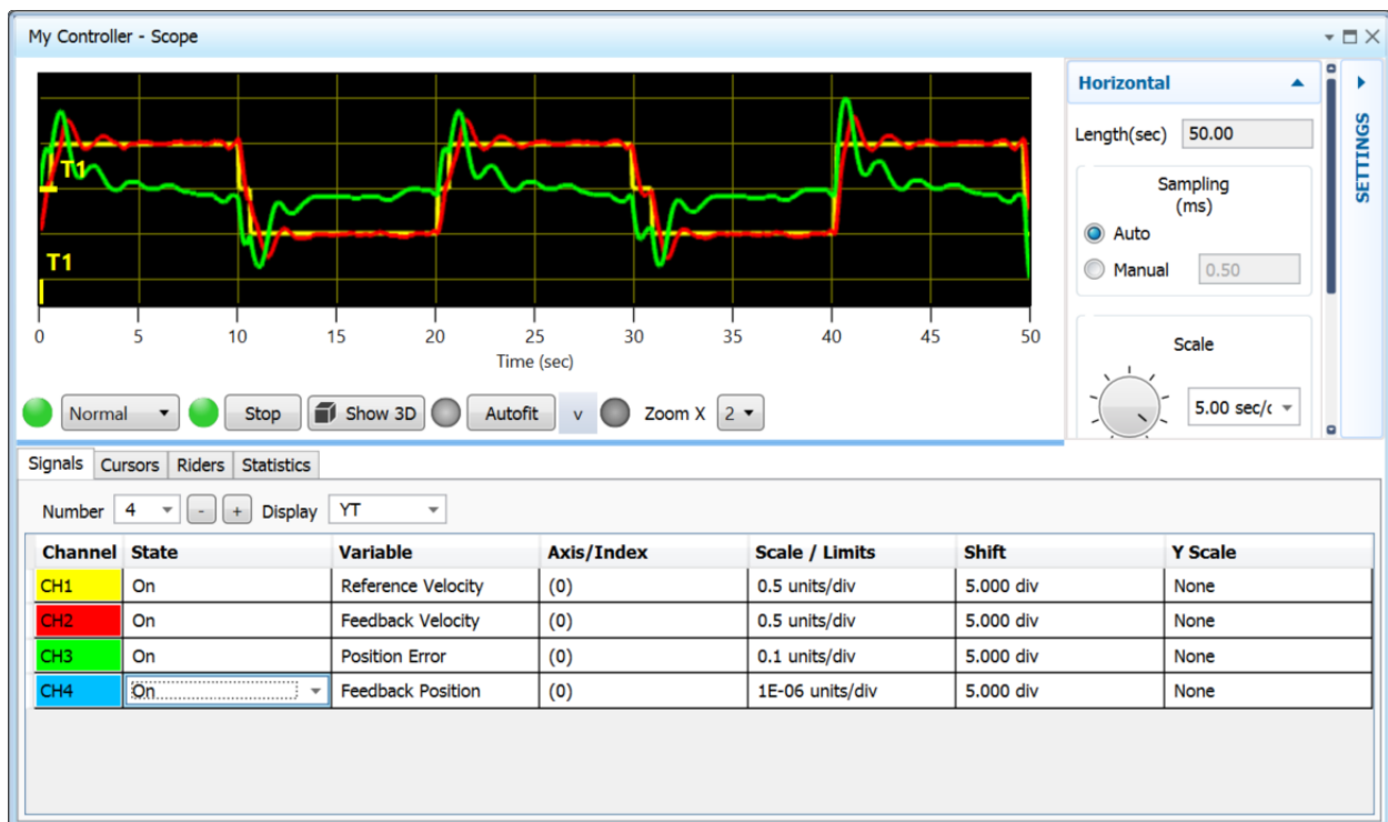
Figure 77: SPiiPlus Scope output giving validity to tuning parameters during a Motion Manager back and forth move. Feedback velocity follows reference velocity and a low, steady-state position error. Note the scale of the position error is 0.1 units/division.
