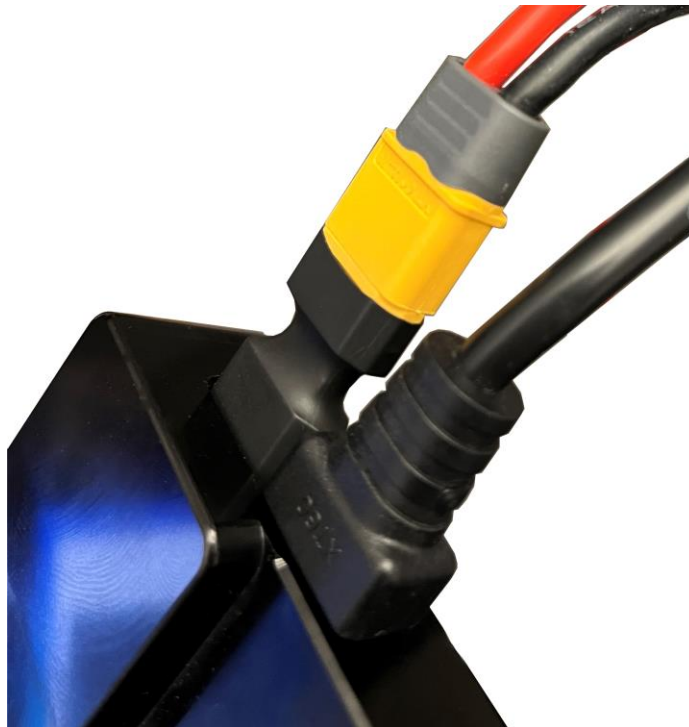
Figure 28: A female-to-female XT60 extender plugged into the Instrument Panel's Power Port 3.
