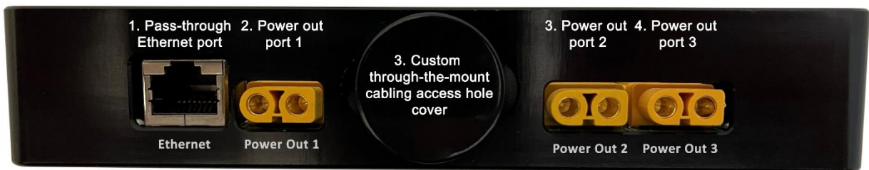
Figure 44: The Paramount MX Instrument Panel components.
