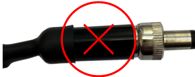
Figure 37: Note that the MKS 5000 PSU plug is not compatible with the MKS 6000.
