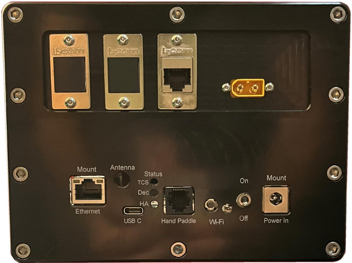
Figure 23: The Paramount ME electronics housing and thorough-the-mount panel.
