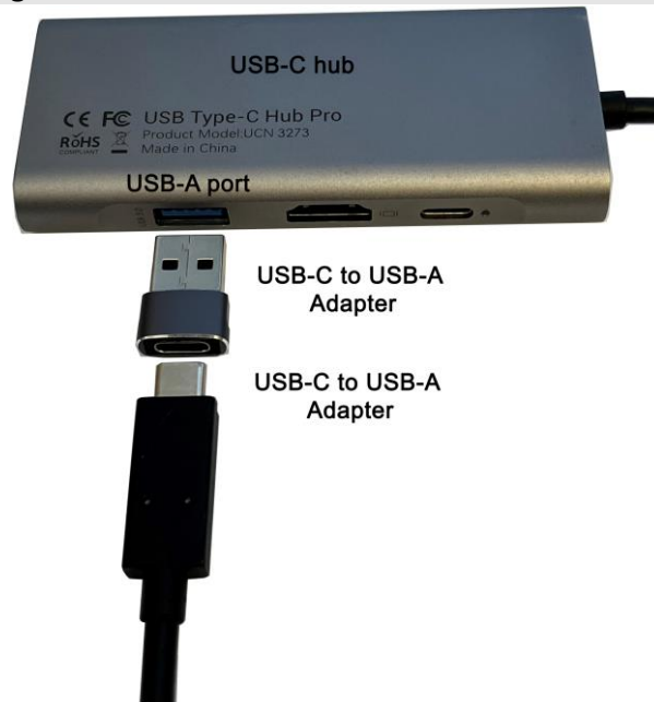
Figure 31: USB cable with USB-C to USB-A adapter.
