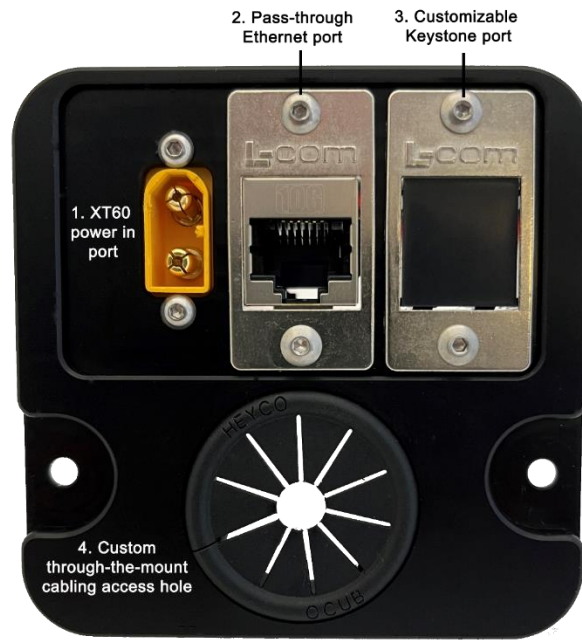
Figure 45: The through-the-mount panel components.
