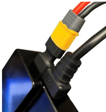
Figure 47: A female-to-female XT60 extender plugged into the Instrument Panel's Power Port 3.
