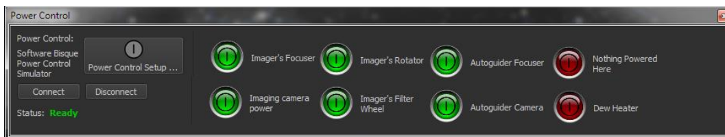
TheSky Imaging Edition's Power Control window provides software-based power port control.
